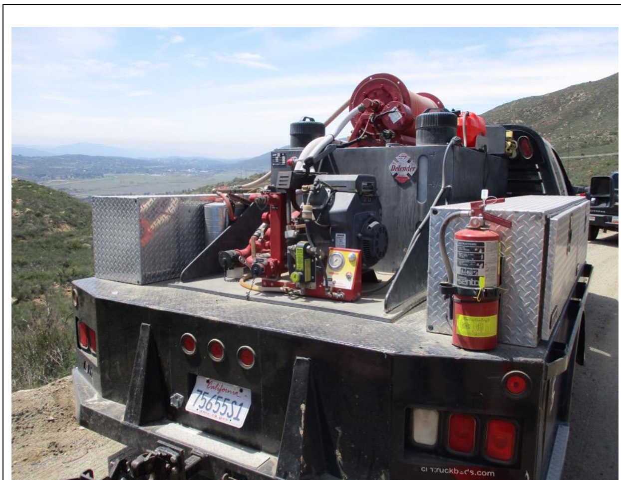
Photo 3: The required fire tools (such as 5 gallon backpack pump, Pulaski, round point shovel, and 2A10BC fire extinguisher) were observed on-site in accordance with the CFPPP, MM FF-1, MM BIO-6, and APM HAZ-4.
